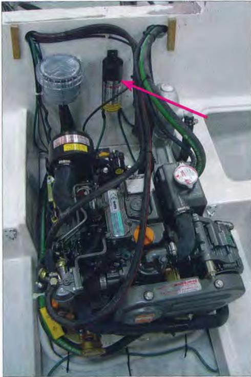
The boat's builder (C&C Fiberglass Components, Bristol, Rhode Island) mounted a standard fail-safe isolator (from Dairyland Electric, Stoughton, Wisconsin) in the engine compartment, where it is easily accessible for necessary periodic testing.
